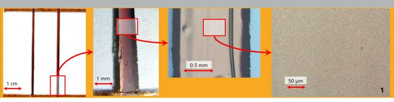
Copper ink lines converted to conductors by flame treatment next page:
